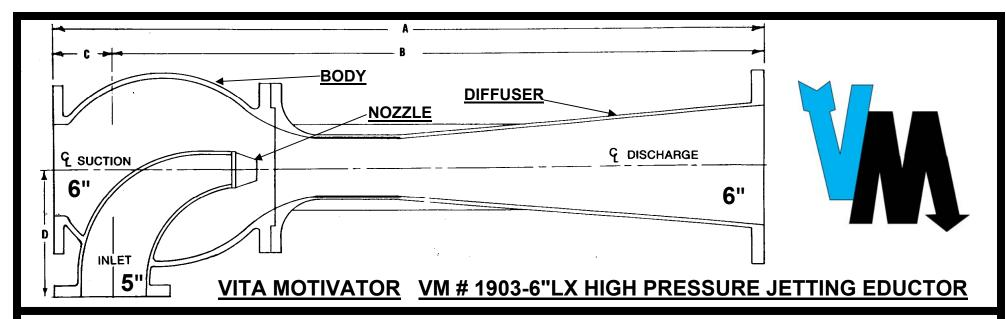
MaterialsProject DataBody & DiffuserBronze ASTM B62Service:NozzleMonelApplication:
